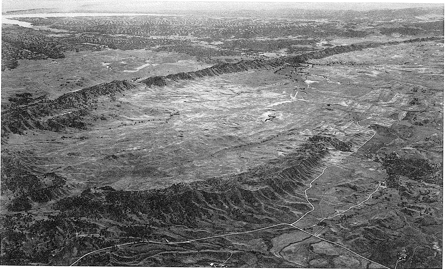
View to the southeast over Newville Reservoir area, with Black Butte Reservoir at upper left. Newville Dam site is the low opening in the right third of the prominent Rocky Ridge, where trees fan out into the valley. A diversion canal from Thomes Creek would enter the valley through the same gap that the road now travels, in the right of the photograph.
